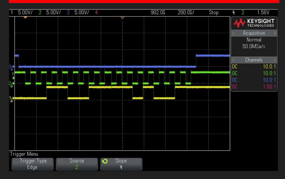
During testing and at the end of this project, the majority of our requirements have been successfully met. Our design uses a standard USB, and it tests open, short and over-voltage conditions. Unfortunately, we were unsuccessful in getting our DAC to work properly, as it outputs a constant voltage of ~1.3V. (For the oscilloscope traces above - Blue: Chip select, Green: System clock, Yellow: Data line 70\*F Testcase)
